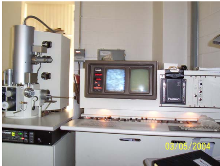
Figure 3.5 Spectrometer Fitted with Scanning Electron Microscope (HITACHI S-800)
